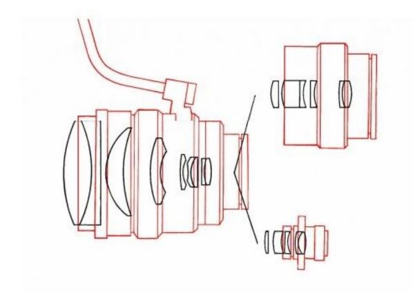
**PENTOVAR 16 - KOMBI** is a variable focal length lens, allowing you to set each focal length in the range from 15 to 120 mm. The lens consists of one set socket and two interchangeable lenses.
