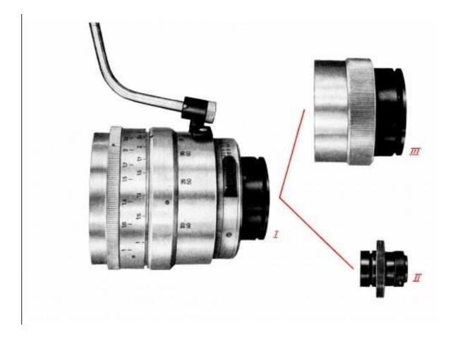
Setting the focal length. The rear lens, small or larger, is screwed clockwise into the rear of the main lens, but the contact surfaces must be absolutely free of dust.
