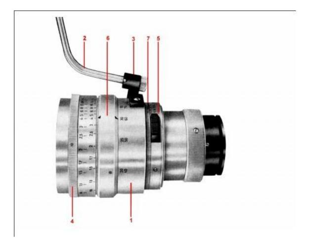
Scales of focal length, distance and apertures are marked with black and red on the appropriate setting rings. The black numbers refer to the combination I - II / f = 15 - 60 mm, the red numbers mean values suitable for the combination I - III / f = 30-120 mm. Ring 6 is provided with arrows for scale f=focal point and E distance.
