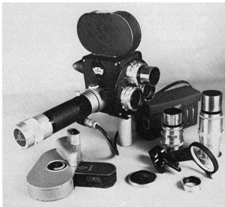
Fig. 4: Accessories Collection standard motor with single- frame transmission Cassette with coding device Cover for motor bayonet original Zeiss battery 80 mm and 135 mm support bridge for telephoto lenses and adapter for Praktica lenses
