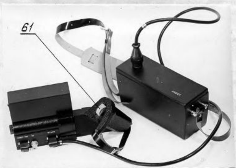
Fig. 13. Direct current electric drive with stable speed of 29EPSS
